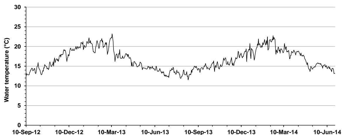
Figure 5.7. Water temperatures profile in slab tanks over the entire on-farm trial at Coastal Seafarms (11/9/12 - 26/6/14; 653 d).
